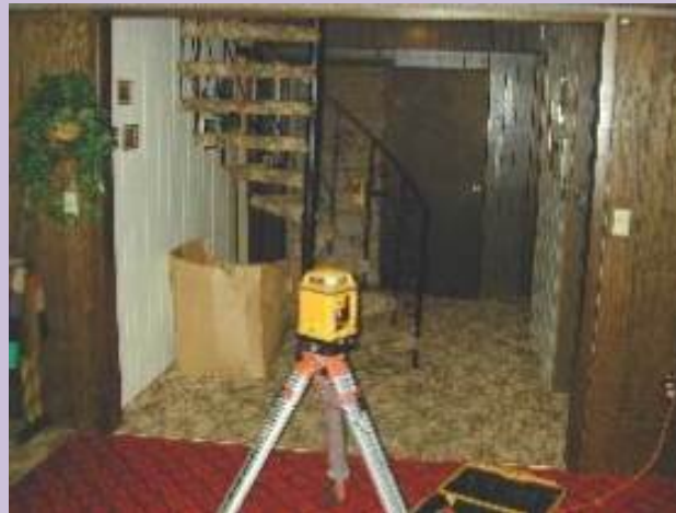
Continuous laser level monitoring to detect minute structural movement from drilling & grouting.
