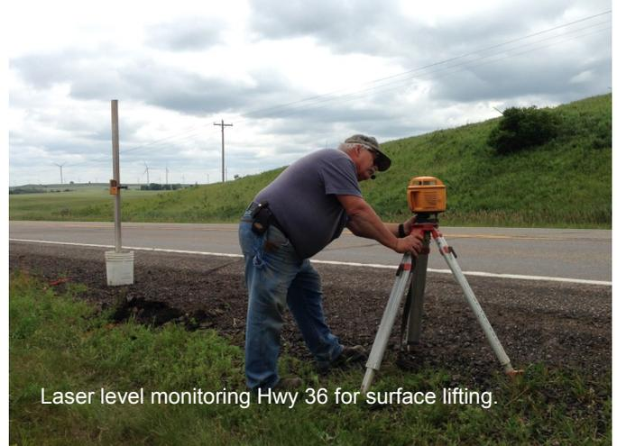
Laser level monitoring Hwy 36 for surface lifting.
