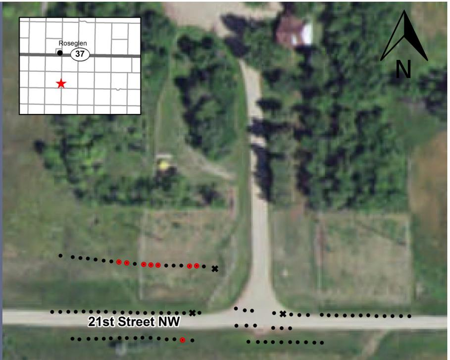
The east—west road is 21<sup>st</sup> Street NW. Each **black dot** represents one drill hole that encountered solid coal. **Red dots** are holes that intercepted mine workings and were cased for future work. A **black x** indicates a hole that was abandoned before reaching the coal.
