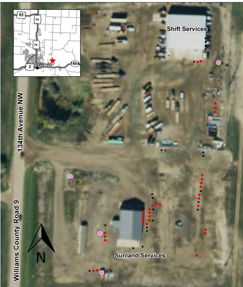
Williams County Road 9 runs north and south. Shift Services occupies the building to the north. The building to the south was formerly occupied by Sunland Services. Each **black dot** represents one drill hole that encountered solid coal. **Red dots** are holes that intercepted mine workings and were cased for future work. Sinkholes are represented by **pink dots**.
