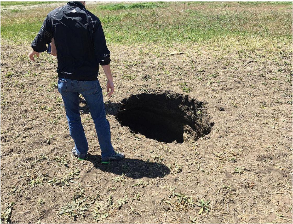
This shows AML employee, Jordan Burns, inspecting a sinkhole on a cropland field near New Salem. Although small in diameter at the surface, beneath the surface this dangerous sinkhole was 12 feet long, five feet wide and five feet deep.
