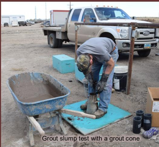
Grout slump test with a grout cone
