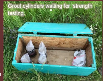
Grout cylinders waiting for strength testing.
