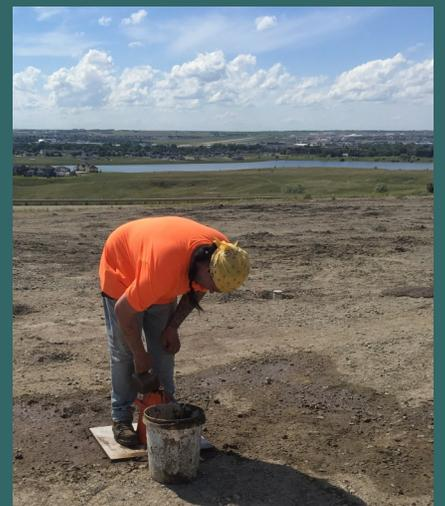
The material tester is doing a slump test on grout at Williston.
