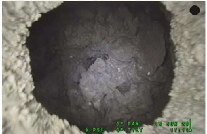
The camera is about to leave the drill hole and enter a void.
