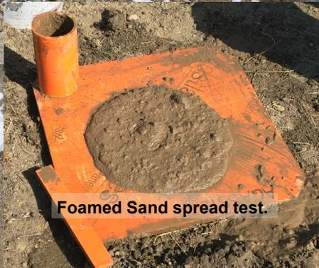
Foamed Sand spread test.
