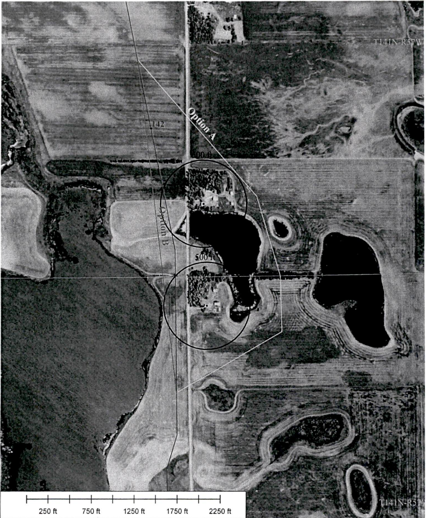
Barnes County, ND Red Line - Keystone Centerline Yellow Line - Option A (+1225') Blue Line - Option B (-15')
