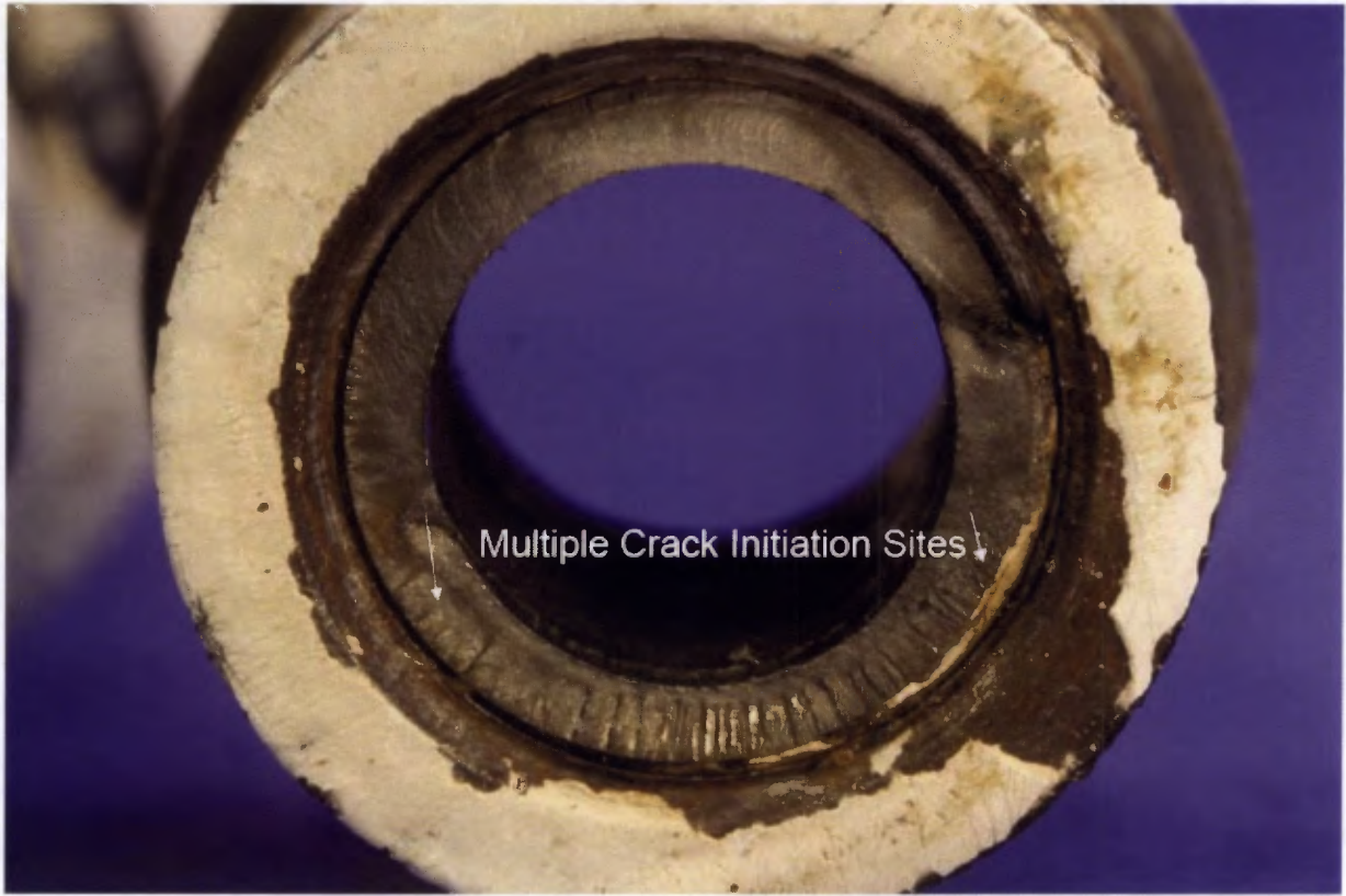
Figure 7: Close-up View of the Failure Surface Defined by Zones 1, 2 &3, As-received
