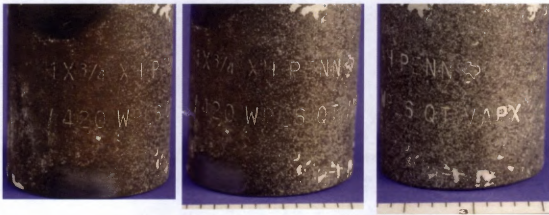
Figure 6: Stamped Markings on Swage Fittings
