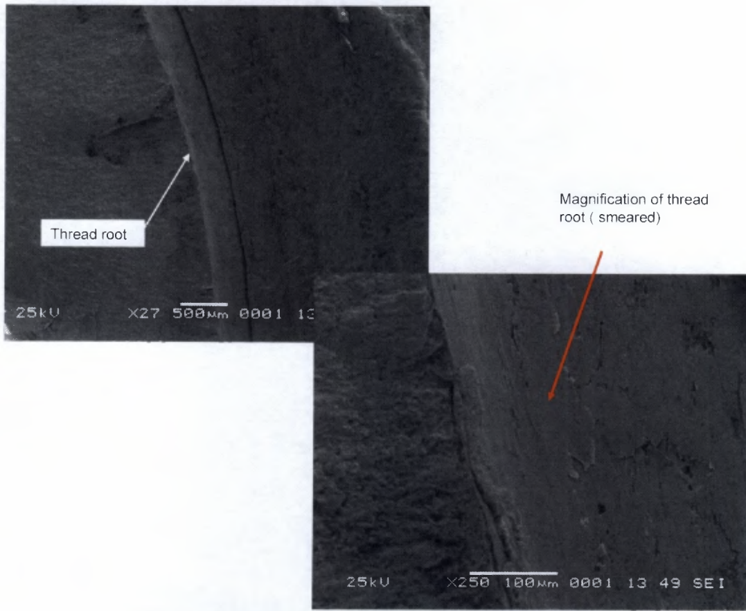
Figure 9: Appearance on the Root of the First Thread
