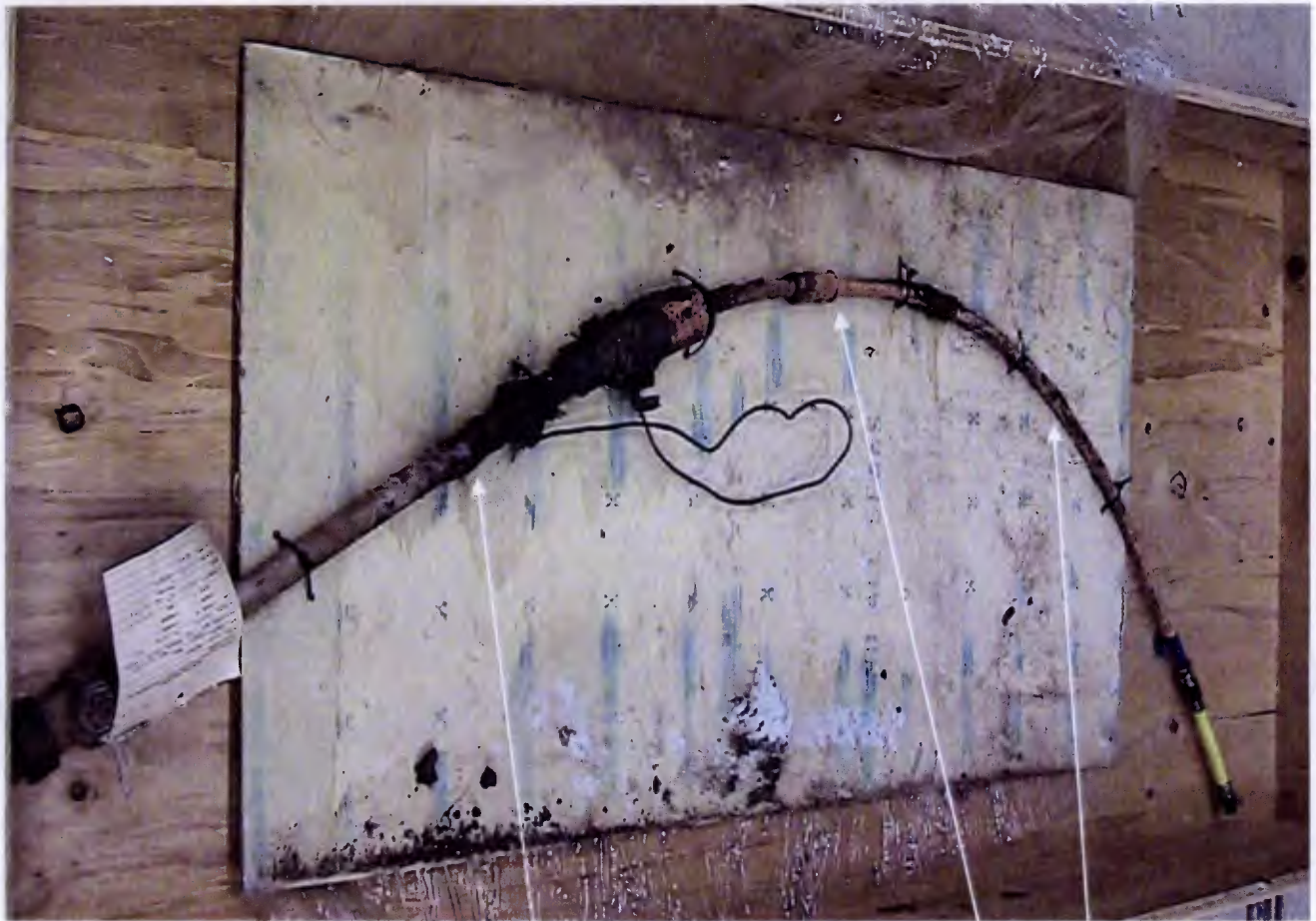
Riser socket coupler service line pipe section sent to CRT Laboratories, Inc.
