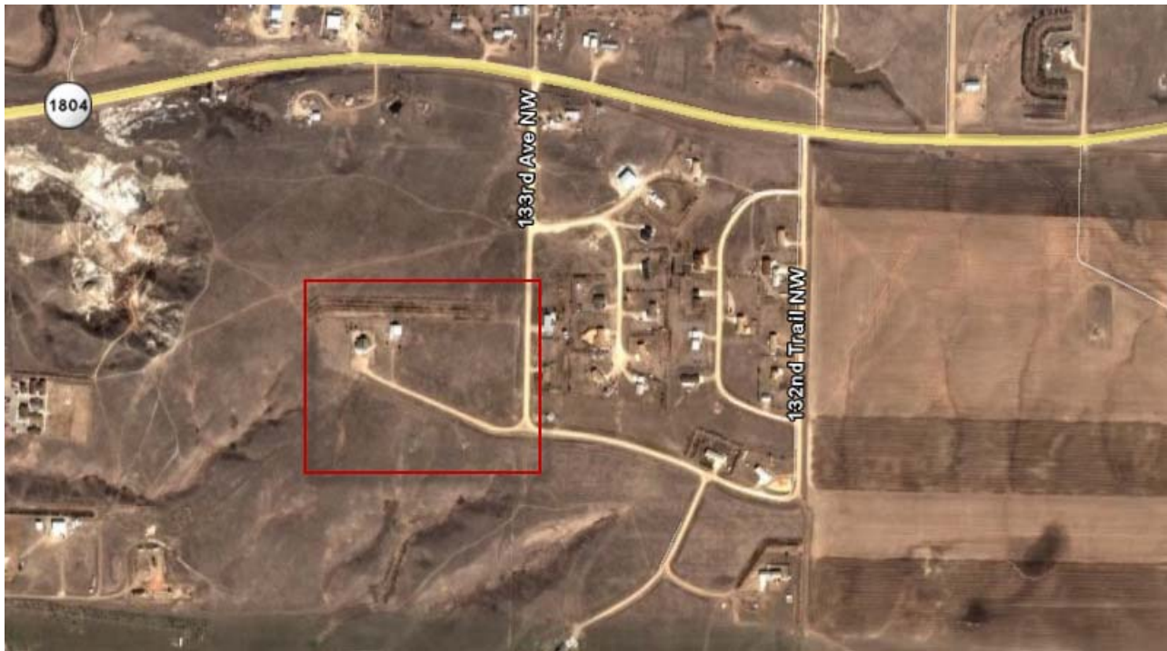
Detail Map 2: proposed drilling and grouting near Scenic East Subdivision, Solberg property, driveway and home; Section 20, T154N, R100W (approx 3 acres disturbance).
