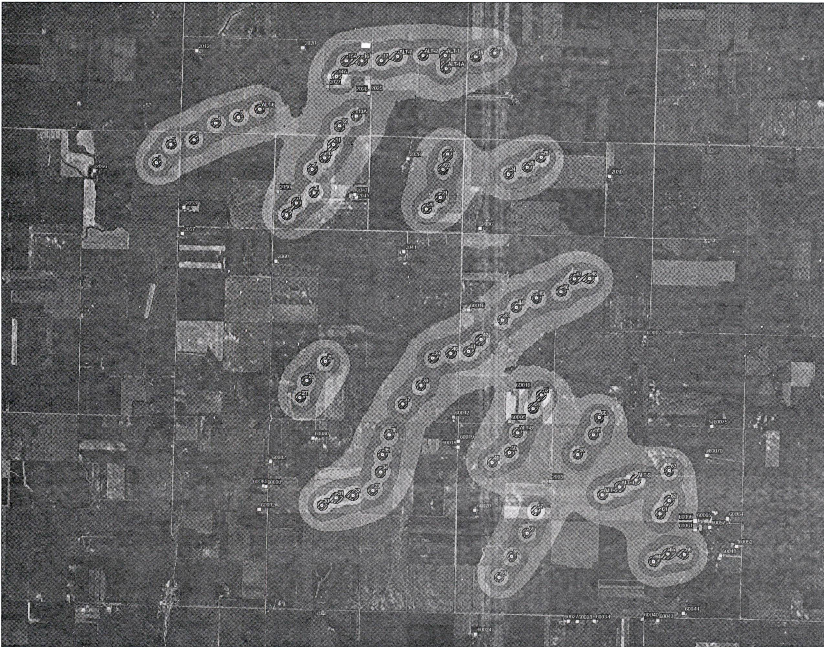
FIGURE 2 RECEIVED SOUND LEVELS WTGS AT CUT-IN
