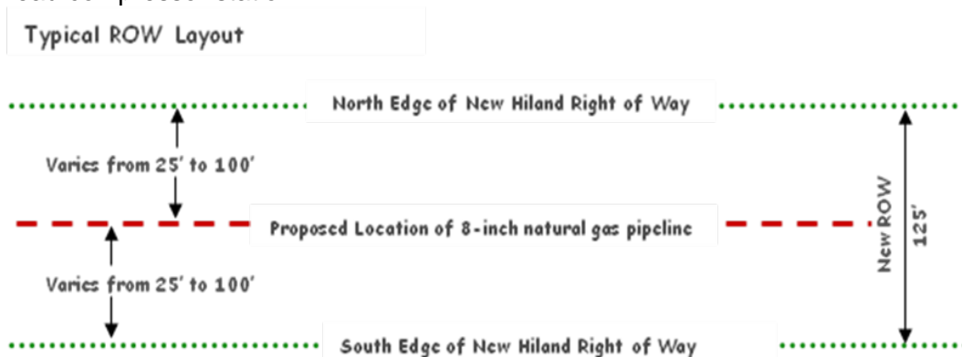
FIGURE 3.B.3 – Typical Right-of-Way Configuration
