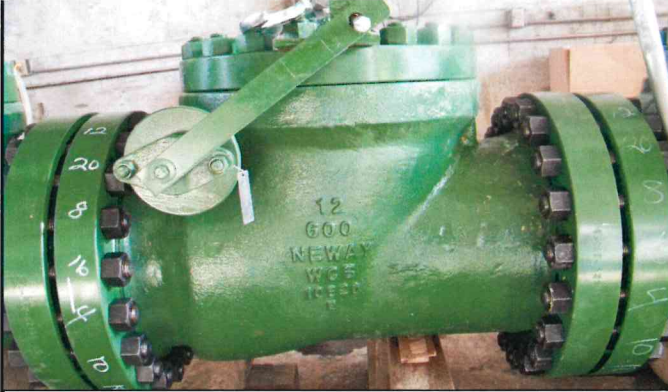
Check valve during HydroTesting
