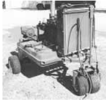
Unit mounts on a four-wheel cart built out of 2-in. sq. tubing. An oversized radiator out of a 3/4-ton pickup cools the engine.
