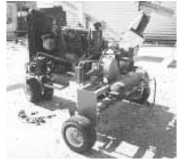
The gearbox is at a right angle to the engine crankshaft instead of in-line so it doesn't take up much room.
