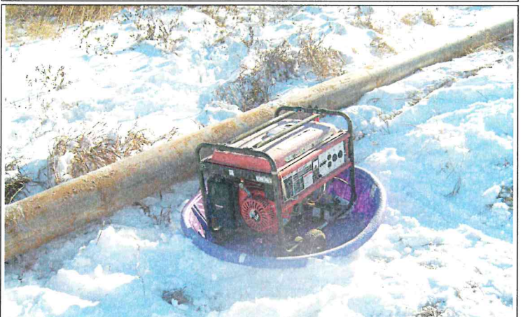
Use of secondary containment structure.
