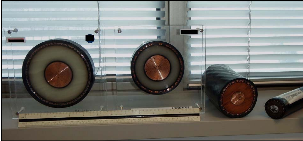
Underground XLPE cables left to right: 345 kV, 138 kV, 69 kV, and distribution
