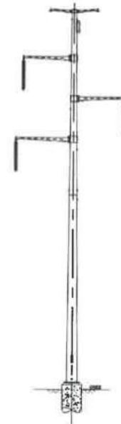
TANGENT STRUCTURE SINGLE POLE - 3ST2
