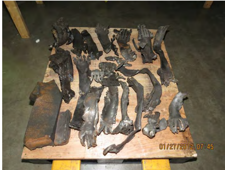
Picture 4: Damaged LP turbine blades.
