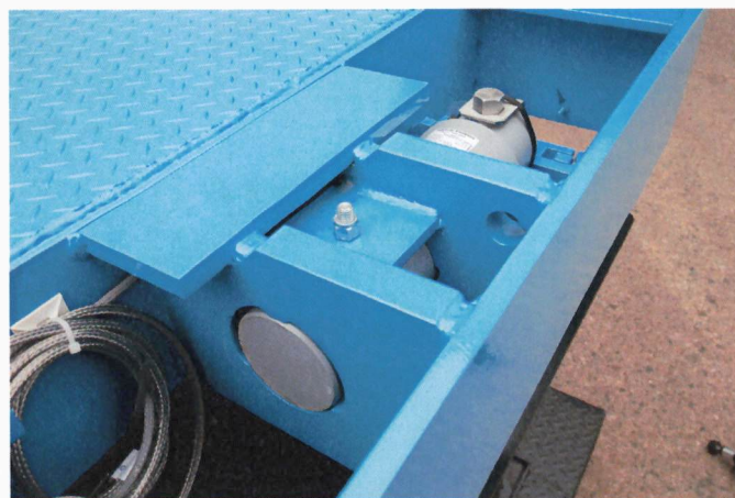
Cover plate removed over the load cell area for easy access and cleaning.
