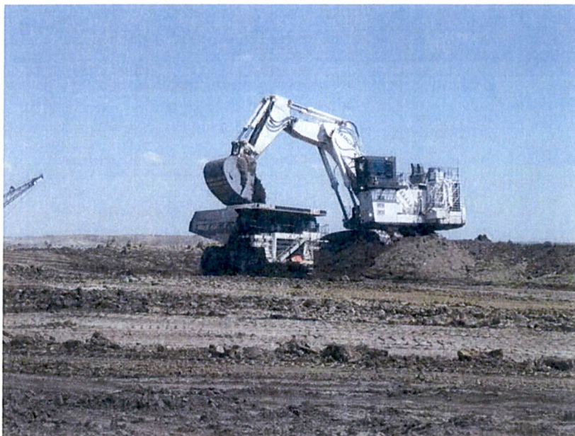
Photo 6: Photo shows 542 truck fleet handling topsoil from a private surface owner. North Dakota rules require the segregation of soil separately from different landowners unless they otherwise agree to mixing. Falkirk is in negotiations with this owner to allow the mixing of topsoil and subsoil removed from his property with soil owned by others.
