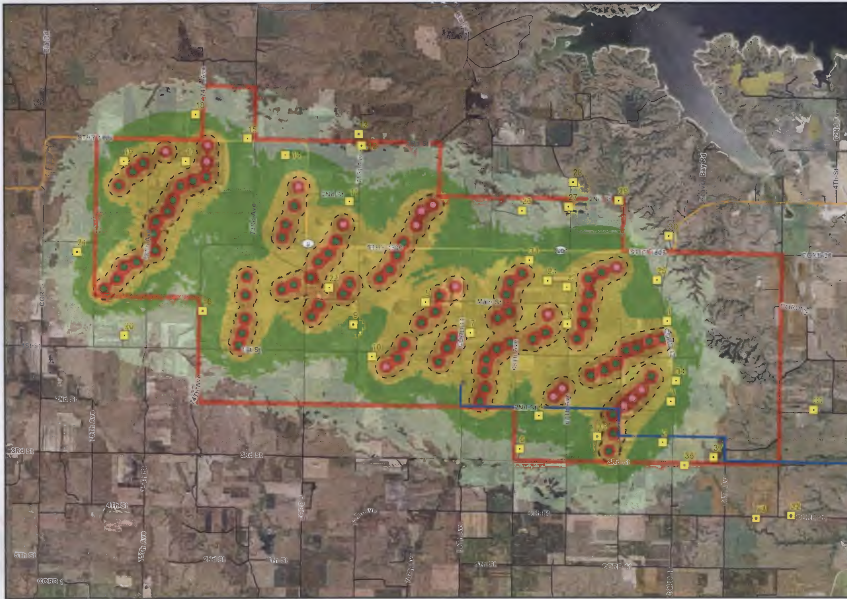
Antelope Hills Wind Project Application for North Dakota Certificate of Site Compatibility Figure 2 Operational Leq Sound Levels under Anomalous Meteorological Conditions - Siemens SWT 2.3-108 Mercer County, ND October 2014
