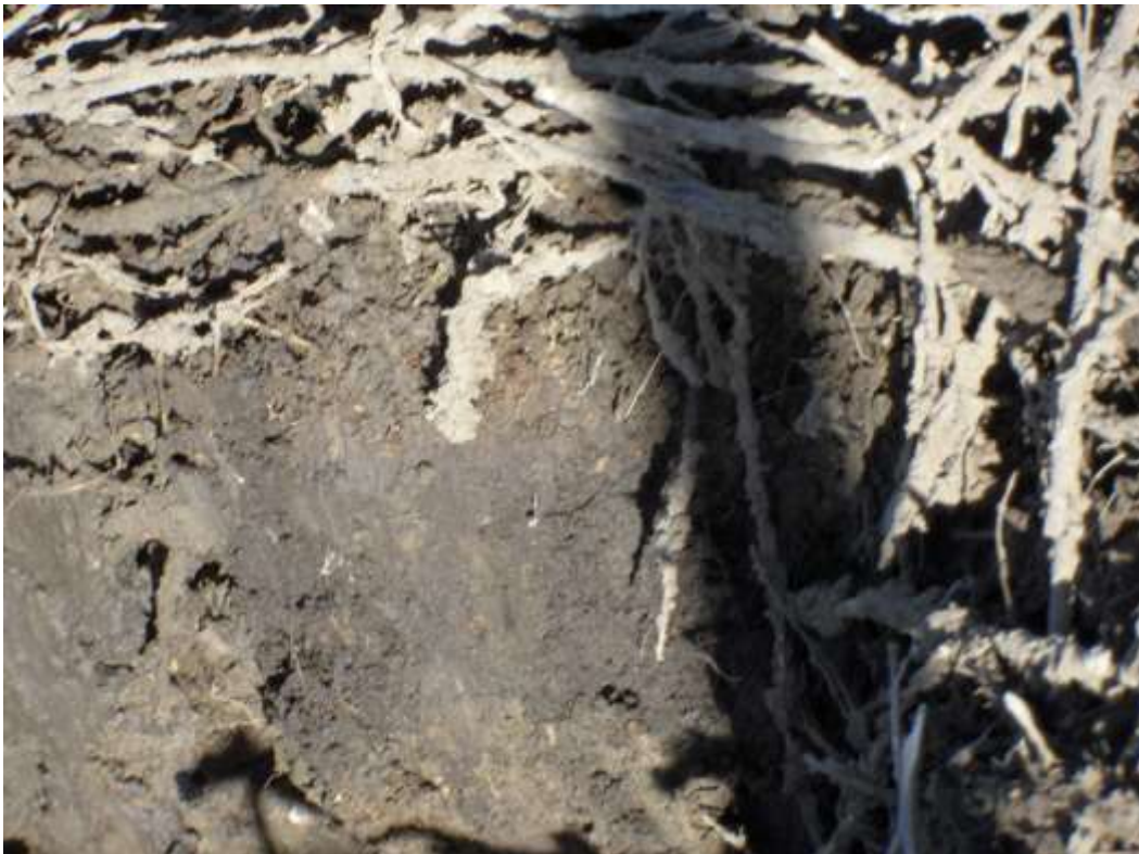
Report Photo #2 "Six (6) Inch Topsoil depth" at GPS Coordinates:
