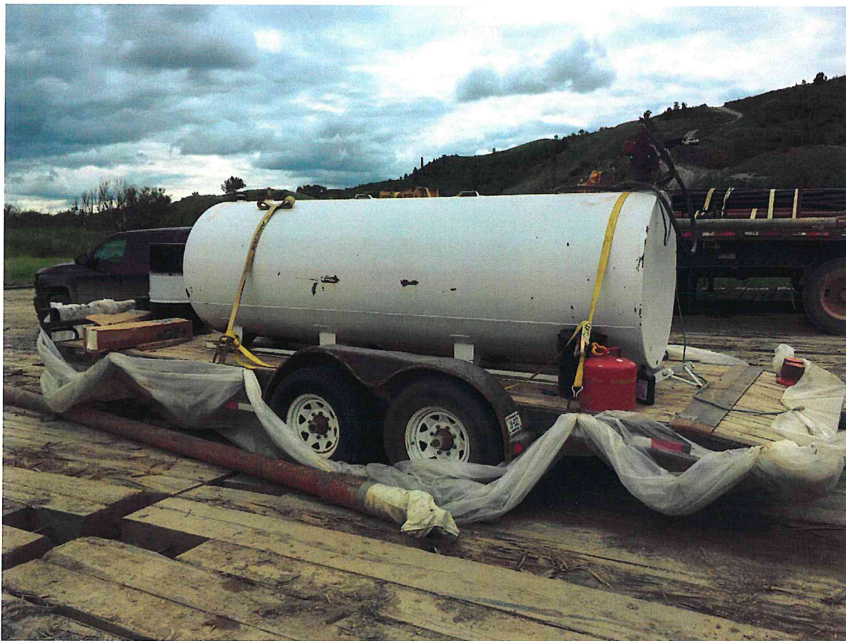
Photo 1 –Inadequate secondary containment at 47.6087°N -102.8765°W
