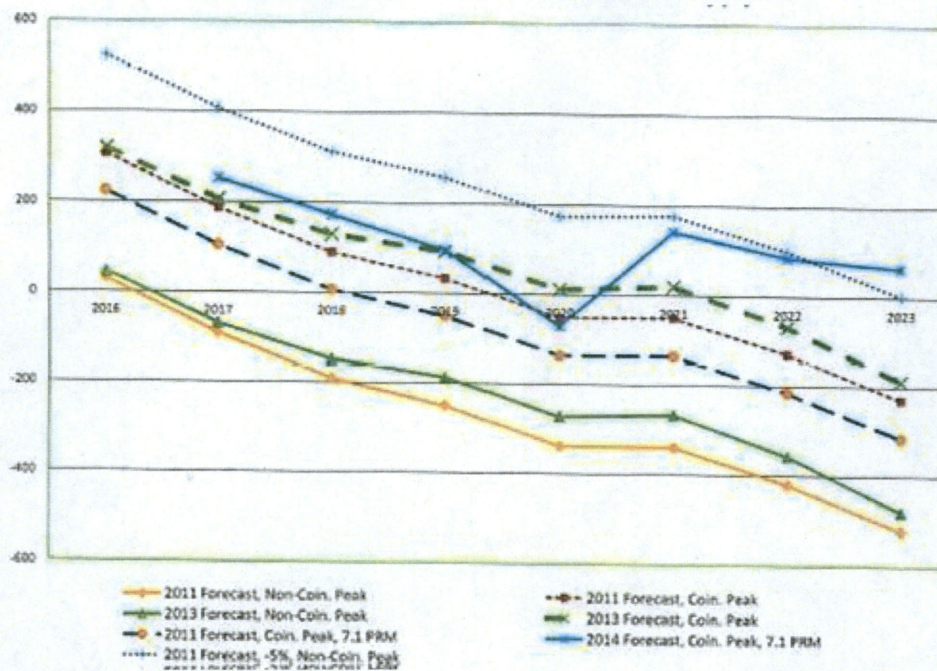
Figure 3: Impact of Coincident and Non-Coincident Peak Methodologies on Resource Plan Need Forecasts
