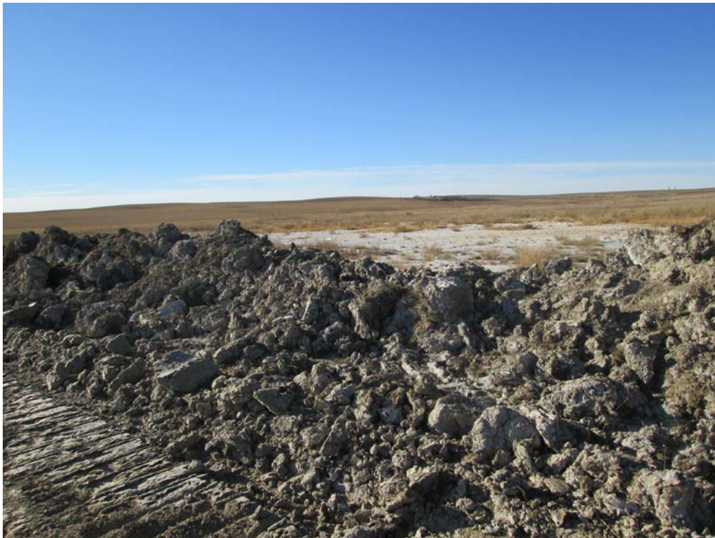
Below: Photo 14 (pt. 210) – Topsoil pile has white crusts. Note white area in background in undisturbed area.
