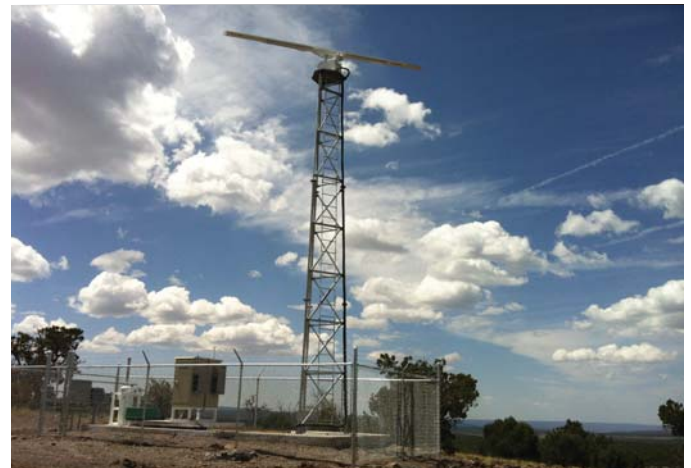
ABOVE: The HARRIER ADLS is typically supplied as a fixed, self-contained skid mounted system for ground based installation. BELOW: HARRIER ADLS web display
