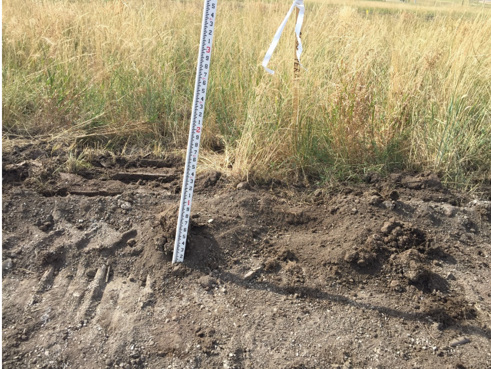
Photo 24: Sta. 126+00 8-9 inches topsoil.
