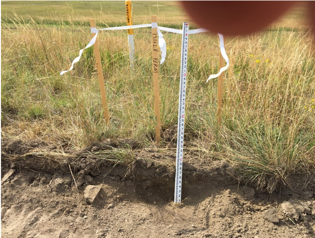
Photo 27: Sta.131+28 8-9 inches of topsoil.
