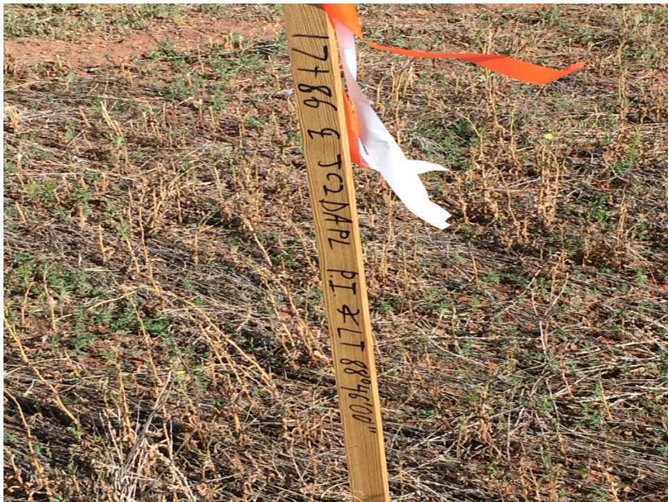
Photo 8: Sta. 17+86 point of intersection angle Lt. 88°46'00"
