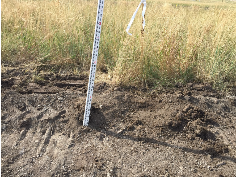
Photo 24: Sta. 126+00 8-9 inches topsoil.
