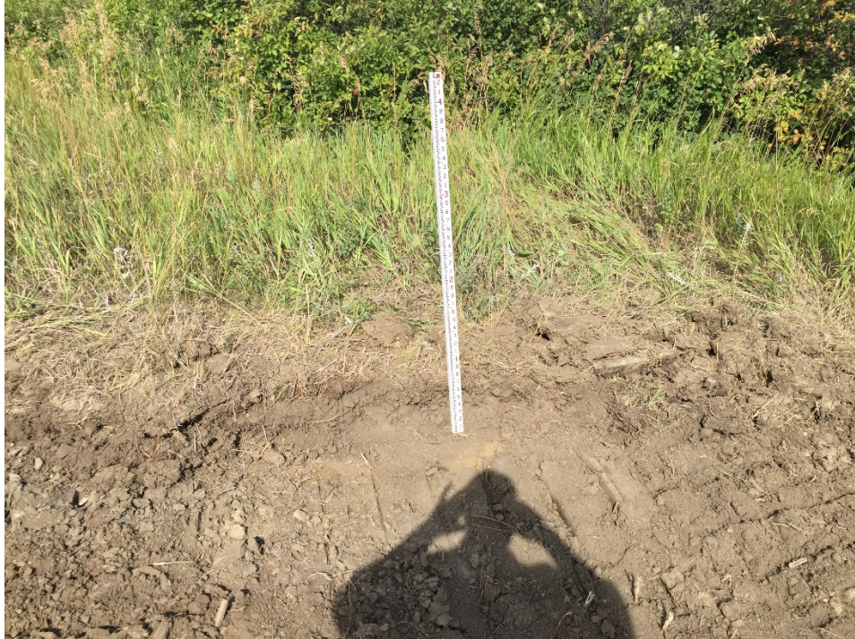
Photo 20: Sta. 108+00, 8-10 inches of topsoil.
