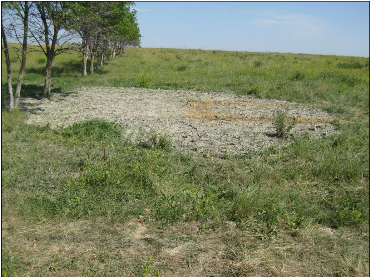
Figure 2. Typical surface expression of a frac-out.
