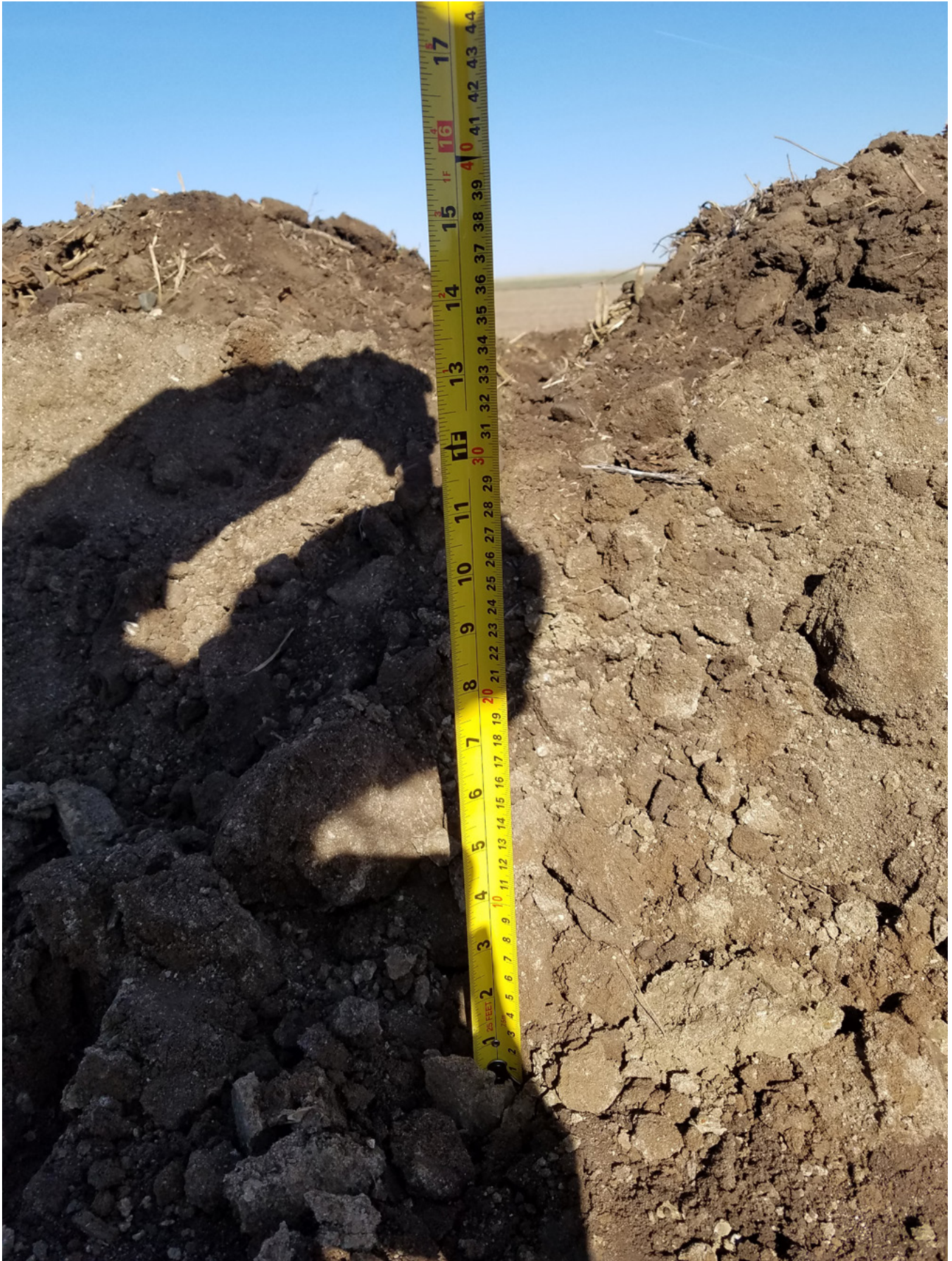
Photo 14 - 12" topsoil depth looking north along the north edge of the pad
