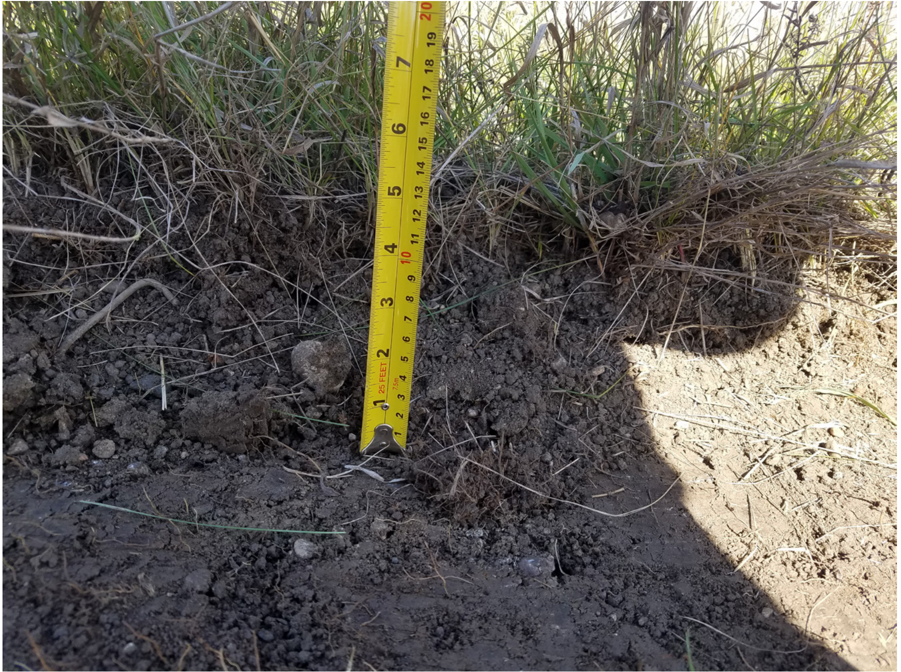
Photo 2 - 3" topsoil depth on the hill south of the southwest fence corner
