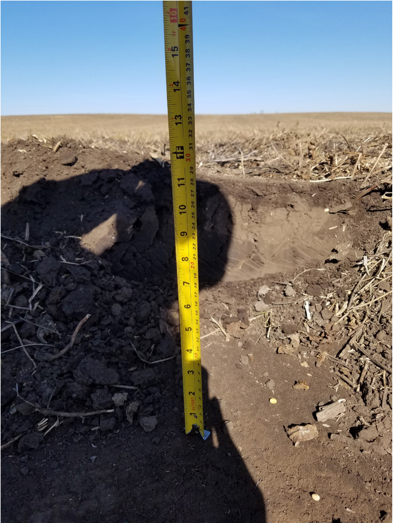
Photo 15 - 10" topsoil depth looking north along north edge at northwest pad corner
