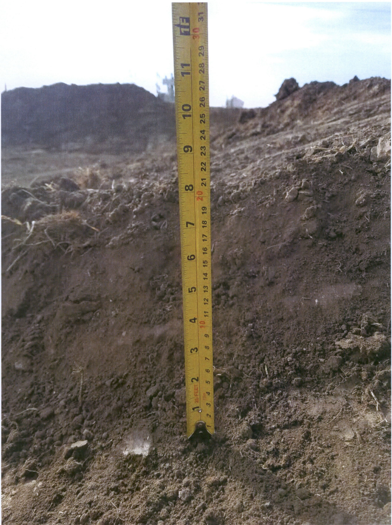
Photo 5 – 7" topsoil replacement depth northwest corner of site
