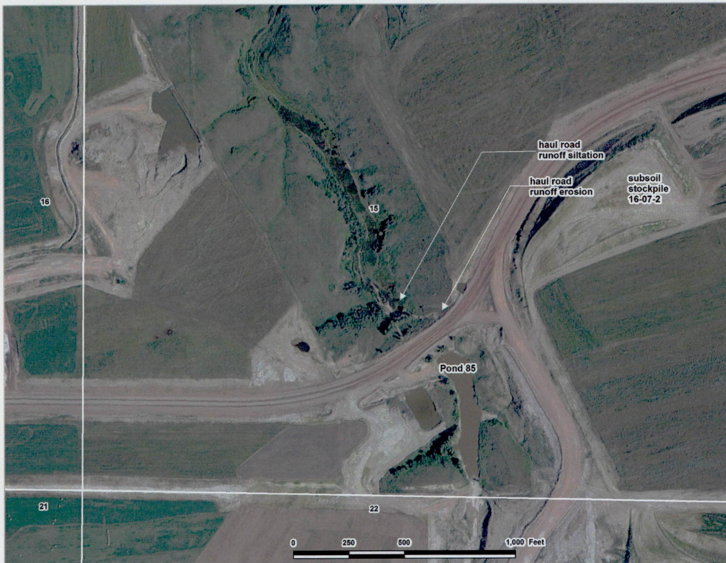
Figure 8. Detailed location of haul road erosion and siltation in the S \frac{1}{2} SW \frac{1}{4} of Section 15 where the Pond 85 embankment functions as the intermittent stream haul road crossing at this location. Also shown in the upper left is Special Variance Zone #7 (spoil stockpile to reclaim Pond 86 and its associated sump). Aerial photography is courtesy of the USDA-NAIP dated August 9, 2016 - see Figure 1 for location.
