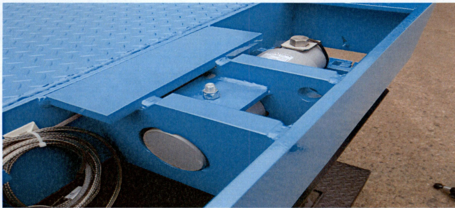
Cover plate removed over the load cell area for easy access and cleaning.
