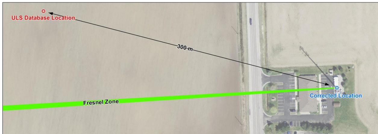
Figure 3: Example of using USGS Orthoimagery to correct erroneous ULS database antenna location
