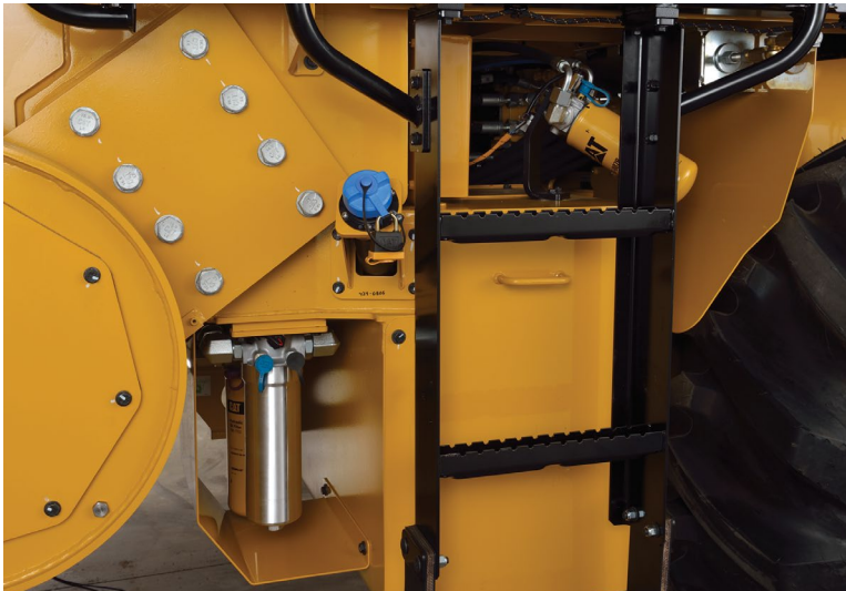
LEFT: Easy access to hydraulic filters and DEF fill port
