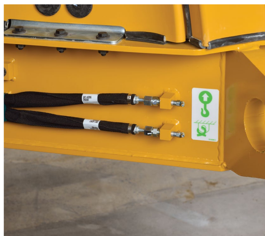
Grouped Remote Grease Fittings
