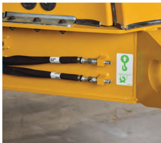
Grouped Remote Grease Fittings
