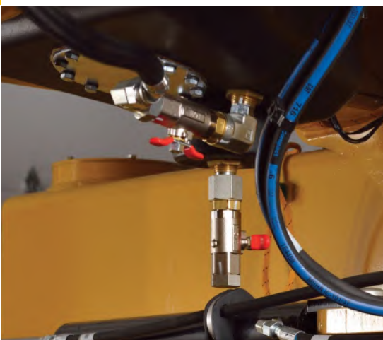
Grouped Drain Valves
