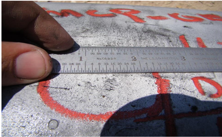
Figure J-4. Example Photograph of SCC Colony Close-up
