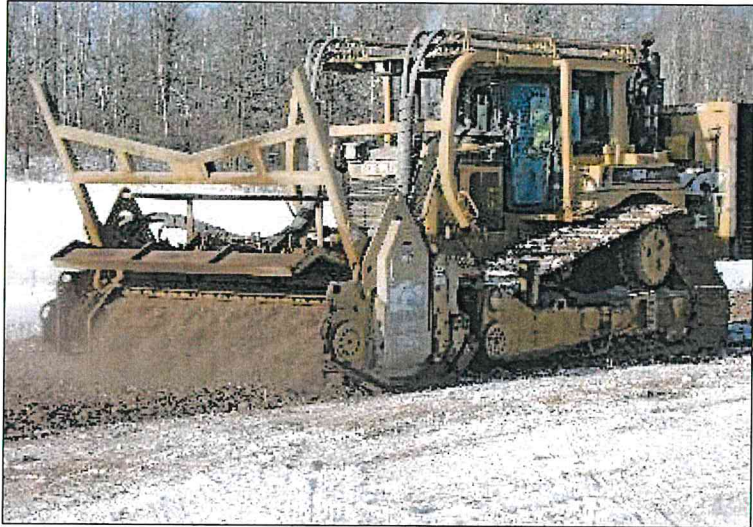
Iron Wolf Breaking up Frozen Topsoil
