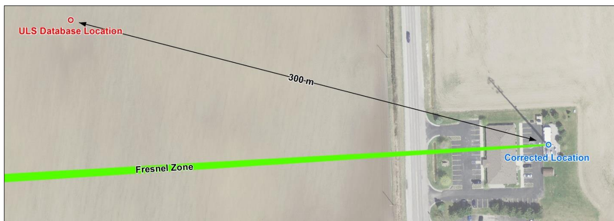
Figure 3: Example of using aerial imagery to correct erroneous ULS database antenna location
