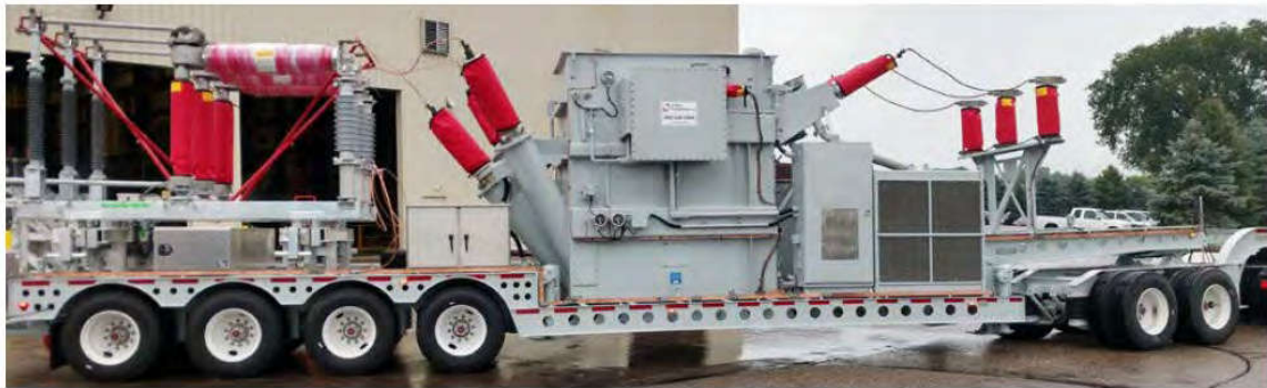
12 13 Figure 7 – Mobile Distribution Substation Example
