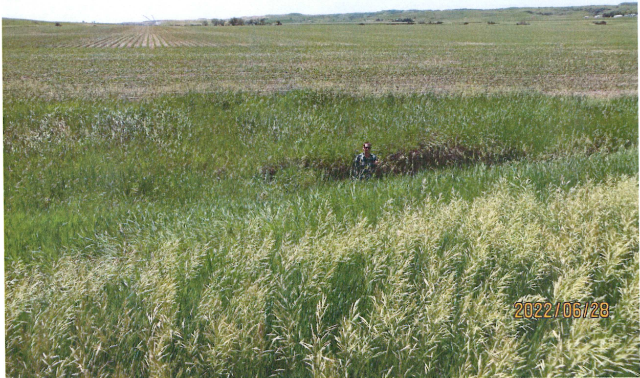
Figure 3. A head cut in the diversion that was approximately 40 feet in length, 6 feet wide, and 3 feet in depth. The inspector standing in the diversion head cut is 6 feet tall. The photo was taken facing south.
