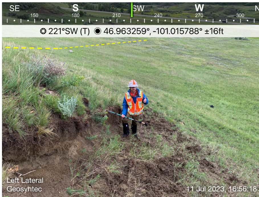
Looking southwest at the left lateral flank of the recently active shallow landslide. The approximate proposed pipeline is located along top left of the image (dashed yellow line). Recent cattle activity had exposed bare soil within the landslide.
