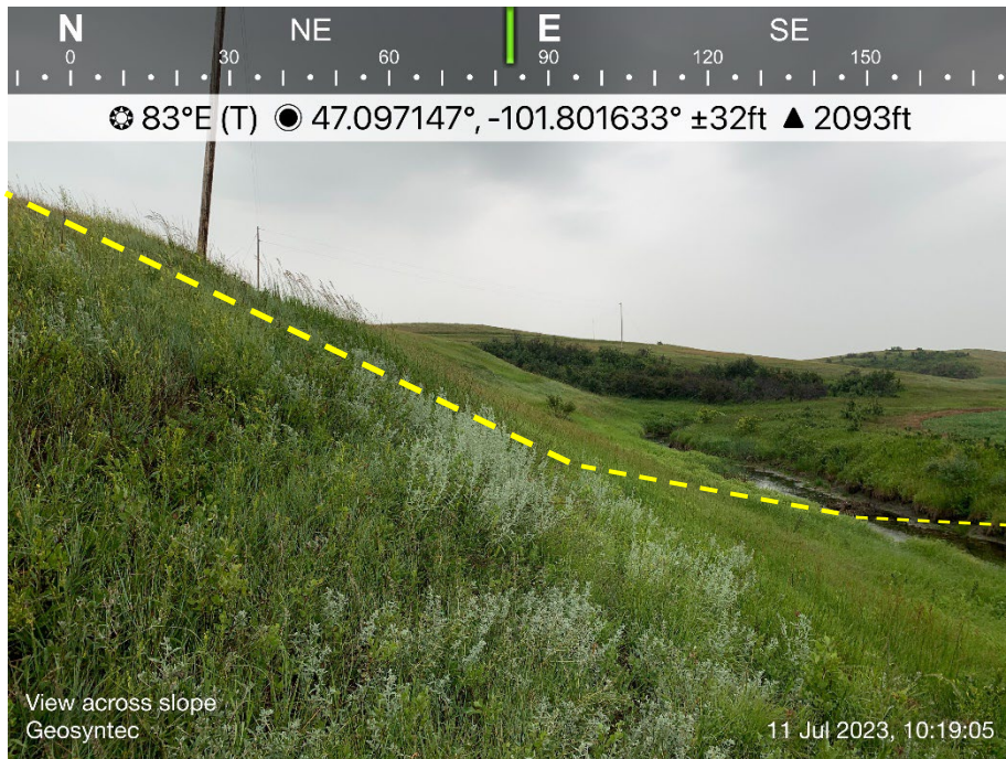
Looking east across the slope in the vicinity NDL-325B (MP 4.6-4.7). The approximate proposed pipeline is located in the center of the image (dashed yellow line). No landslide morphology was observed in the vicinity of the proposed pipeline.
