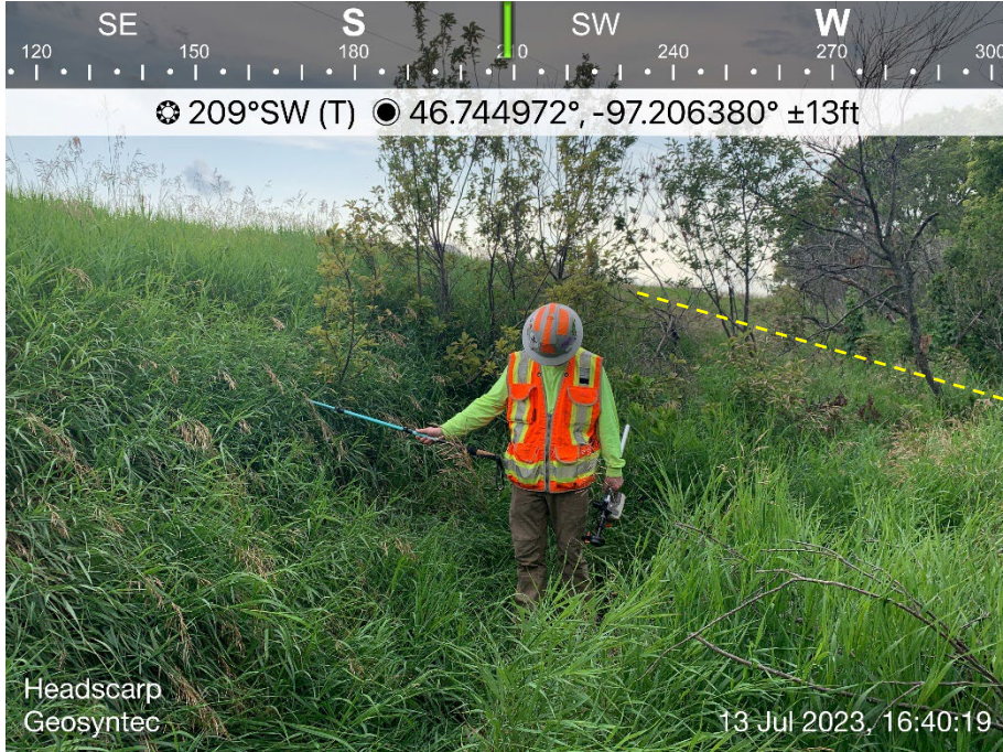
Looking southwest at a possible 3-foot high headscarp crossed by the proposed pipeline centerline. The approximate location of the proposed pipeline centerline is represented by the dashed yellow line.
