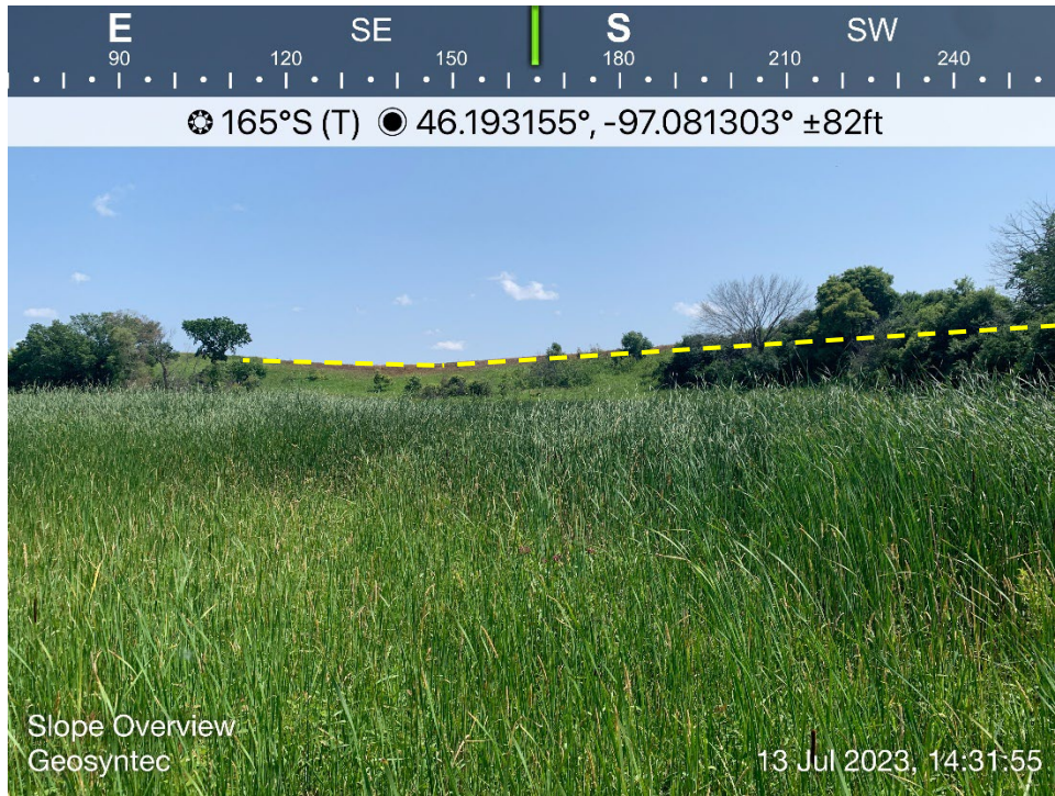
Looking south across the slope in the vicinity NDT-211 (MP 3.5-3.7). The approximate proposed pipeline is located in the center of the image (dashed yellow line). No landslide morphology was observed in the vicinity of the proposed pipeline.
