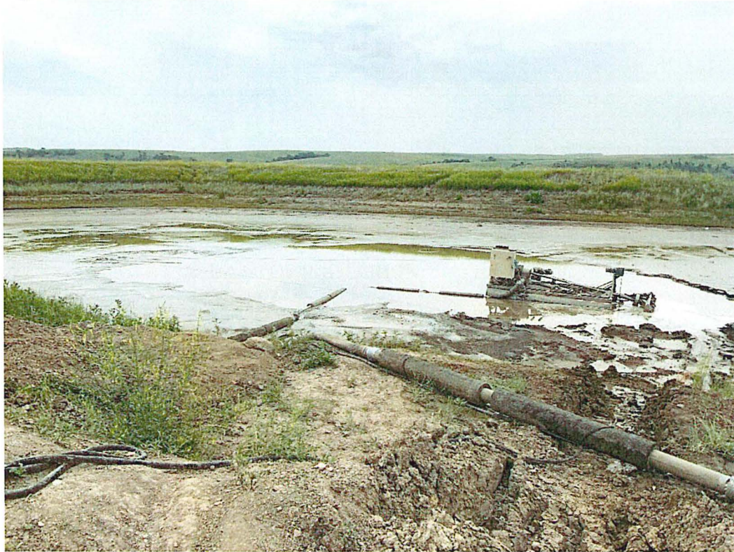
Figure 2. Head cut erosion near the stripping edge in the SW \frac{1}{4} of Section 25.
