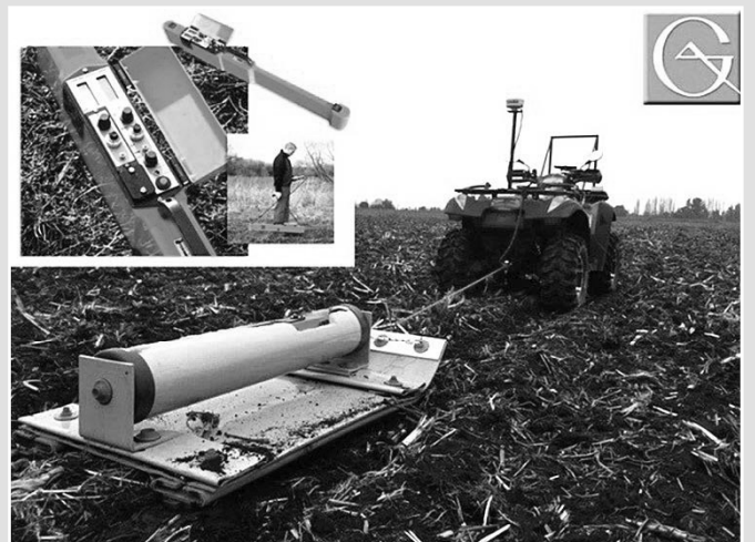
Figure 9. EM38 in use. (Courtesy of Geonics Ltd., Mississauga, Ontario)
