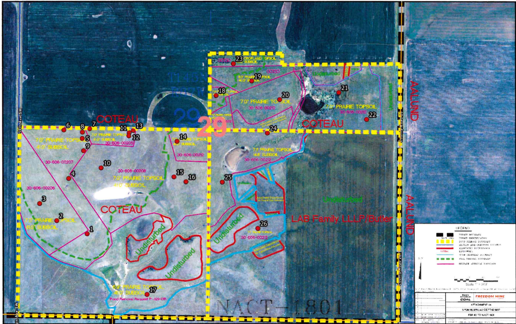
Figure 1. Soil probe locations and numbers for assessing SPGM thickness in Section 29 of Permit NACT-1801. The map depicts grade approval boundaries, required SPGM thickness, and bond release boundaries.
