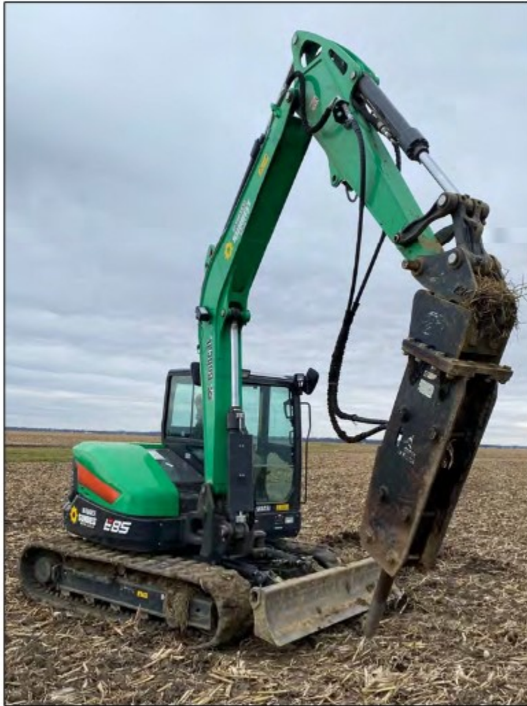
Bobcat E85 mini-excavator fitted with an Okada 1100H hydraulic impact hammer
