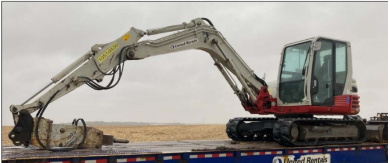
Excavator and Vibratory Hammer used for Pile Installation
