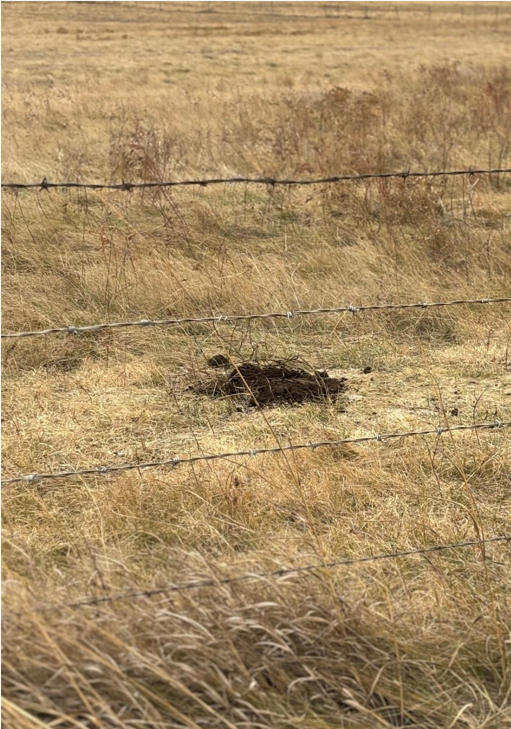
Figure 1 - WP14 – Improperly Finished Borehole
